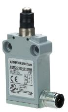
AutomationDirect compact limit switch, metal plunger with dust cap, (1) N.O./(1) N.C. contact(s), snap action, 25mm hole spacing, zinc alloy, (1) 5-pin M12 quick-disconnect, right exit.
