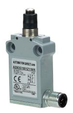
AutomationDirect compact limit switch, metal plunger with dust cap, (1) N.O./(1) N.C. contact(s), snap action, 25mm hole spacing, zinc alloy, 5-pin M12 quick-disconnect, right exit.
