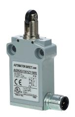
AutomationDirect compact limit switch, metal plunger with nylon cross roller, (1) N.O./(1) N.C. contact(s), snap action, 25mm hole spacing, zinc alloy, (1) 5-pin M12 quick-disconnect, right exit.
