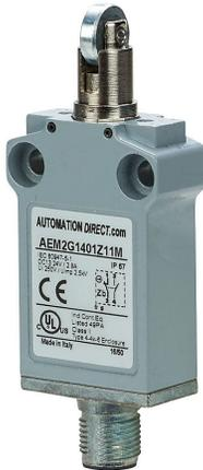
AutomationDirect compact limit switch, metal plunger with metal cross roller, (1) N.O./(1) N.C. contact(s), snap action, 25mm hole spacing, zinc alloy, (1) 5-pin M12 quick-disconnect, bottom exit.
