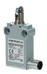
AutomationDirect compact limit switch, metal plunger with metal cross roller, (1) N.O./(1) N.C. contact(s), snap action, 25mm hole spacing, zinc alloy, (1) 5-pin M12 quick-disconnect, right exit.
