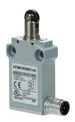
AutomationDirect compact limit switch, metal plunger with nylon roller, (1) N.O./(1) N.C. contact(s), snap action, 25mm hole spacing, zinc alloy, (1) 5-pin M12 quick-disconnect, right exit.
