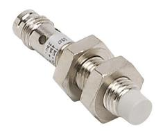
Micro Detectors inductive proximity sensor, tubular, 8mm diameter x 40mm body, nickel-plated brass housing, PNP, N.O. output, 4mm sensing distance, non-flush, 3 kHz switching frequency, IP67, 3-pin M8 quick-disconnect.
