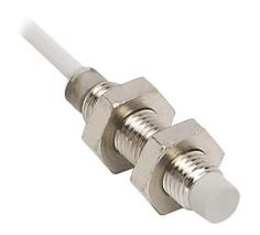
Micro Detectors inductive proximity sensor, tubular, 8mm diameter x 35.5mm body, nickel-plated brass housing, PNP, N.O. output, 4mm sensing distance, non-flush, 3 kHz switching frequency, IP67, pigtail.
