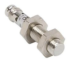
Micro Detectors inductive proximity sensor, tubular, 8mm diameter x 40mm body, nickel-plated brass housing, PNP, N.O. output, 2mm sensing distance, flush, 3 kHz switching frequency, IP67, 3-pin M8 quick-disconnect.
