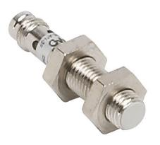
Micro Detectors inductive proximity sensor, tubular, 8mm diameter x 40mm body, nickel-plated brass housing, PNP, N.O. output, 2mm sensing distance, flush, 3 kHz switching frequency, IP67, 3-pin M8 quick-disconnect.
