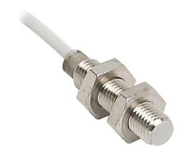
Micro Detectors inductive proximity sensor, tubular, 8mm diameter x 35.5mm body, nickel-plated brass housing, PNP, N.O. output, 2mm sensing distance, flush, 3 kHz switching frequency, IP67, pigtail.
