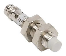
Micro Detectors inductive proximity sensor, tubular, 8mm diameter x 40mm body, nickel-plated brass housing, NPN, N.O. output, 4mm sensing distance, non-flush, 3 kHz switching frequency, IP67, 3-pin M8 quick-disconnect.
