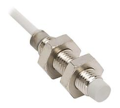
Micro Detectors inductive proximity sensor, tubular, 8mm diameter x 35.5mm body, nickel-plated brass housing, NPN, N.O. output, 4mm sensing distance, non-flush, 3 kHz switching frequency, IP67, pigtail.
