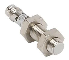
Micro Detectors inductive proximity sensor, tubular, 8mm diameter x 40mm body, nickel-plated brass housing, NPN, N.O. output, 2mm sensing distance, flush, 3 kHz switching frequency, IP67, 3-pin M8 quick-disconnect.
