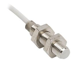
Micro Detectors inductive proximity sensor, tubular, 8mm diameter x 35.5mm body, nickel-plated brass housing, NPN, N.O. output, 2mm sensing distance, flush, 3 kHz switching frequency, IP67, pigtail.
