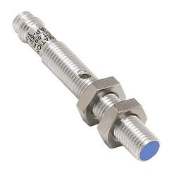
AutomationDirect inductive proximity sensor, tubular, 8mm diameter x 60mm body, chrome-plated brass housing, PNP, N.O. output, 3mm sensing distance, semi-flush, 1 kHz switching frequency, IP67, 3-pin M8 quick-disconnect.
