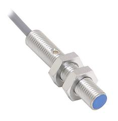
AutomationDirect inductive proximity sensor, tubular, 8mm diameter x 45mm body, chrome-plated brass housing, PNP, N.O. output, 3mm sensing distance, semi-flush, 1 kHz switching frequency, IP67, pigtail.
