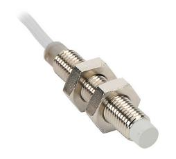
Micro Detectors inductive proximity sensor, tubular, 8mm diameter x 45mm body, nickel-plated brass housing, PNP, N.O. output, 4mm sensing distance, non-flush, 3 kHz switching frequency, IP67, pigtail.
