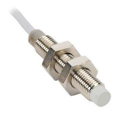
Micro Detectors inductive proximity sensor, tubular, 8mm diameter x 45mm body, nickel-plated brass housing, PNP, N.O. output, 4mm sensing distance, non-flush, 3 kHz switching frequency, IP67, pigtail.
