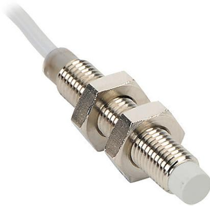
Micro Detectors inductive proximity sensor, tubular, 8mm diameter x 45mm body, nickel-plated brass housing, PNP, N.O. output, 4mm sensing distance, non-flush, 3 kHz switching frequency, IP67, pigtail.
