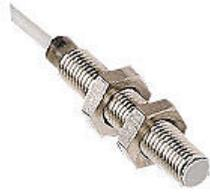
Micro Detectors inductive proximity sensor, tubular, 8mm diameter x 45mm body, nickel-plated brass housing, PNP, N.O. output, 2mm sensing distance, flush, 3 kHz switching frequency, IP67, pigtail.
