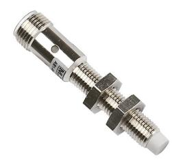
Micro Detectors inductive proximity sensor, tubular, 8mm diameter x 60mm body, nickel-plated brass housing, PNP, N.O. output, 2.5mm sensing distance, non-flush, 2.5 kHz switching frequency, IP67, 4-pin M12 quick-disconnect.
