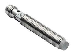
Micro Detectors inductive proximity sensor, tubular, 8mm diameter x 50mm body, nickel-plated brass housing, PNP, N.O. output, 2.5mm sensing distance, non-flush, 2.5 kHz switching frequency, IP67, 3-pin M8 quick-disconnect.
