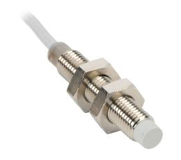
Micro Detectors inductive proximity sensor, tubular, 8mm diameter x 45mm body, nickel-plated brass housing, PNP, N.O. output, 2.5mm sensing distance, non-flush, 2.5 kHz switching frequency, IP67, pigtail.
