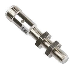
Micro Detectors inductive proximity sensor, tubular, 8mm diameter x 60mm body, nickel-plated brass housing, PNP, N.O. output, 1.5mm sensing distance, flush, 3 kHz switching frequency, IP67, 4-pin M12 quick-disconnect.
