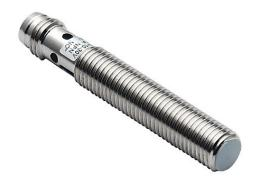
Micro Detectors inductive proximity sensor, tubular, 8mm diameter x 50mm body, nickel-plated brass housing, PNP, N.O. output, 1.5mm sensing distance, flush, 3 kHz switching frequency, IP67, 3-pin M8 quick-disconnect.
