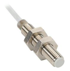
Micro Detectors inductive proximity sensor, tubular, 8mm diameter x 45mm body, nickel-plated brass housing, PNP, N.O. output, 1.5mm sensing distance, flush, 3 kHz switching frequency, IP67, pigtail.
