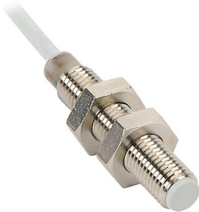
Micro Detectors inductive proximity sensor, tubular, 8mm diameter x 45mm body, nickel-plated brass housing, PNP, N.O. output, 1.5mm sensing distance, flush, 3 kHz switching frequency, IP67, pigtail.
