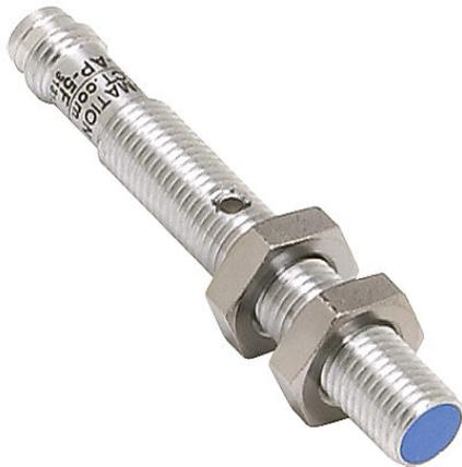
AutomationDirect inductive proximity sensor, tubular, 8mm diameter x 60mm body, chrome-plated brass housing, NPN, N.O. output, 3mm sensing distance, semi-flush, 1 kHz switching frequency, IP67, 3-pin M8 quick-disconnect.
