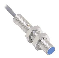
AutomationDirect inductive proximity sensor, tubular, 8mm diameter x 45mm body, chrome-plated brass housing, NPN, N.O. output, 3mm sensing distance, semi-flush, 1 kHz switching frequency, IP67, pigtail.
