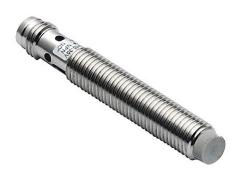
Micro Detectors inductive proximity sensor, tubular, 8mm diameter x 50mm body, nickel-plated brass housing, NPN, N.O. output, 4mm sensing distance, non-flush, 3 kHz switching frequency, IP67, 3-pin M8 quick-disconnect.
