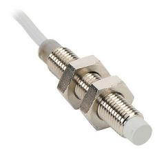
Micro Detectors inductive proximity sensor, tubular, 8mm diameter x 45mm body, nickel-plated brass housing, NPN, N.O. output, 4mm sensing distance, non-flush, 3 kHz switching frequency, IP67, pigtail.
