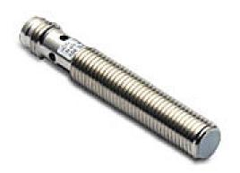
Micro Detectors inductive proximity sensor, tubular, 8mm diameter x 50mm body, nickel-plated brass housing, NPN, N.O. output, 2mm sensing distance, flush, 3 kHz switching frequency, IP67, 3-pin M8 quick-disconnect.
