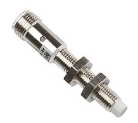
Micro Detectors inductive proximity sensor, tubular, 8mm diameter x 60mm body, nickel-plated brass housing, NPN, N.O. output, 2.5mm sensing distance, non-flush, 2.5 kHz switching frequency, IP67, 4-pin M12 quick-disconnect.
