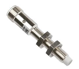
Micro Detectors inductive proximity sensor, tubular, 8mm diameter x 60mm body, nickel-plated brass housing, NPN, N.O. output, 2.5mm sensing distance, non-flush, 2.5 kHz switching frequency, IP67, 4-pin M12 quick-disconnect.
