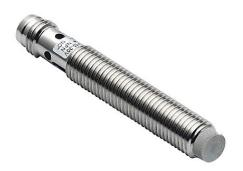
Micro Detectors inductive proximity sensor, tubular, 8mm diameter x 50mm body, nickel-plated brass housing, NPN, N.O. output, 2.5mm sensing distance, non-flush, 2.5 kHz switching frequency, IP67, 3-pin M8 quick-disconnect.
