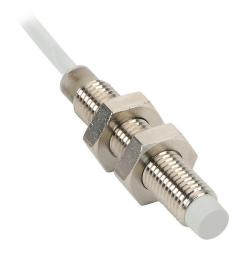
Micro Detectors inductive proximity sensor, tubular, 8mm diameter x 45mm body, nickel-plated brass housing, NPN, N.O. output, 2.5mm sensing distance, non-flush, 2.5 kHz switching frequency, IP67, pigtail.
