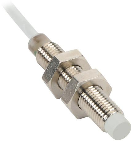
Micro Detectors inductive proximity sensor, tubular, 8mm diameter x 45mm body, nickel-plated brass housing, NPN, N.O. output, 2.5mm sensing distance, non-flush, 2.5 kHz switching frequency, IP67, pigtail.
