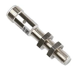
Micro Detectors inductive proximity sensor, tubular, 8mm diameter x 60mm body, nickel-plated brass housing, NPN, N.O. output, 1.5mm sensing distance, flush, 3 kHz switching frequency, IP67, 4-pin M12 quick-disconnect.
