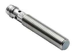
Micro Detectors inductive proximity sensor, tubular, 8mm diameter x 50mm body, nickel-plated brass housing, NPN, N.O. output, 1.5mm sensing distance, flush, 3 kHz switching frequency, IP67, 3-pin M8 quick-disconnect.
