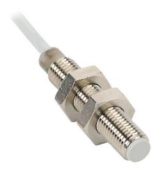
Micro Detectors inductive proximity sensor, tubular, 8mm diameter x 45mm body, nickel-plated brass housing, NPN, N.O. output, 1.5mm sensing distance, flush, 3 kHz switching frequency, IP67, pigtail.
