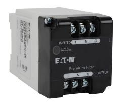
Eaton Aegis series powerline filter, 240 VAC, 1-phase, 5A, 35mm DIN rail mount, EMI/RFI filtering, LED indication, UL Type 2, screw terminals, 5kA SCCR.
