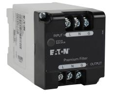
Eaton Aegis series powerline filter, 240 VAC, 1-phase, 3A, 35mm DIN rail mount, EMI/RFI filtering, LED indication, UL Type 2, screw terminals, 5kA SCCR.
