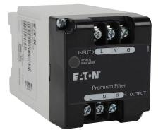
Eaton Aegis series powerline filter, 240 VAC, 1-phase, 1A, 35mm DIN rail mount, EMI/RFI filtering, LED indication, UL Type 2, screw terminals, 5kA SCCR.
