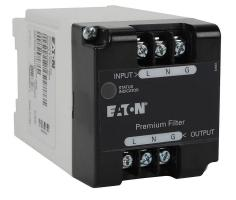
Eaton Aegis series powerline filter, 120 VAC, 1-phase, 5A, 35mm DIN rail mount, EMI/RFI filtering, LED indication, UL Type 2, screw terminals, 5kA SCCR.
