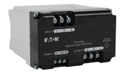
Eaton Aegis series powerline filter, 240 VAC, 1-phase, 15A, 35mm DIN rail mount, EMI/RFI filtering, LED indication, UL Type 2, SPDT alarm, screw terminals, 5kA SCCR.
