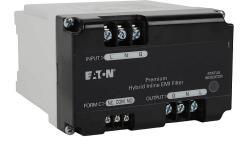
Eaton Aegis series powerline filter, 120 VAC, 1-phase, 15A, 35mm DIN rail mount, EMI/RFI filtering, LED indication, UL Type 2, SPDT alarm, screw terminals, 5kA SCCR.
