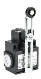
AchieVe IEC limit switch, side rotary adjustable lever with 18mm nylon roller, 90-degree adjustable head, (1) N.O./(1) N.C. contact(s), snap action, 20-22mm or 40-42mm hole spacing, plastic, (2) PG11 cable entries with (1) 1/2in NPT adapter.
