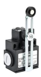
AchieVe IEC limit switch, side rotary 2mm step adjustable lever with 18mm nylon roller, 90-degree adjustable head, (1) N.O./(1) N.C. contact(s), snap action, 20-22mm or 40-42mm hole spacing, plastic, (2) PG11 cable entries with (1) 1/2in NPT adapter.
