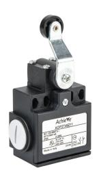
AchieVe IEC limit switch, side rotary lever inward with 18mm nylon roller, 90-degree adjustable head, (1) N.O./(1) N.C. contact(s), snap action, 20-22mm or 40-42mm hole spacing, plastic, (2) PG11 cable entries with (1) 1/2in NPT adapter.
