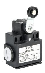
AchieVe IEC limit switch, side rotary lever with 18mm nylon roller, 90-degree adjustable head, (1) N.O./(1) N.C. contact(s), snap action, 20-22mm or 40-42mm hole spacing, plastic, (2) PG11 cable entries with (1) 1/2in NPT adapter.
