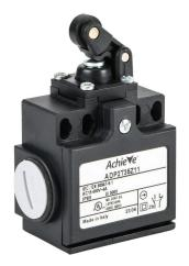
AchieVe IEC limit switch, one-way horizontal lever with metal roller and dust cap, 90-degree adjustable head, (1) N.O./(1) N.C. contact(s), snap action, 20-22mm or 40-42mm hole spacing, plastic, (2) PG11 cable entries with (1) 1/2in NPT adapter.
