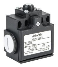
AchieVe IEC limit switch, metal plunger with metal roller and dust cap, 90-degree adjustable head, (1) N.O./(1) N.C. contact(s), snap action, 20-22mm or 40-42mm hole spacing, plastic, (2) PG11 cable entries with (1) 1/2in NPT adapter.
