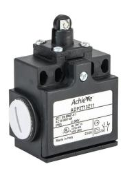
AchieVe IEC limit switch, metal plunger with metal roller, 90-degree adjustable head, (1) N.O./(1) N.C. contact(s), snap action, 20-22mm or 40-42mm hole spacing, plastic, (2) PG11 cable entries with (1) 1/2in NPT adapter.
