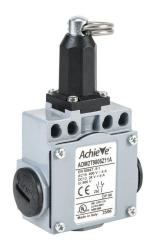
AchieVe IEC limit switch, pull action with ring, 90-degree adjustable head, (1) N.O./(1) N.C. contact(s), snap action, 20-22mm or 40-42mm hole spacing, zinc alloy, (3) 1/2in NPT entries.
