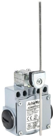
AchieVe IEC limit switch, side rotary adjustable 3mm stainless steel rod, 90-degree adjustable head, (1) N.O./(1) N.C. contact(s), snap action, 20-22mm or 40-42mm hole spacing, zinc alloy, (3) 1/2in NPT entries.
