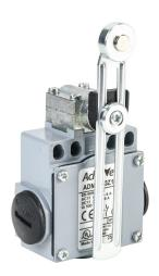
AchieVe IEC limit switch, side rotary adjustable metal lever with 18mm metal roller, 90-degree adjustable head, (1) N.O./(1) N.C. contact(s), snap action, 20-22mm or 40-42mm hole spacing, zinc alloy, (3) 1/2in NPT entries.
